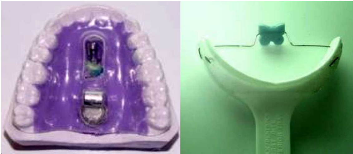
Fig. 3. Prototypes of a vibrostimulation device structured with a micro motor and accessory for lingual exercises.
