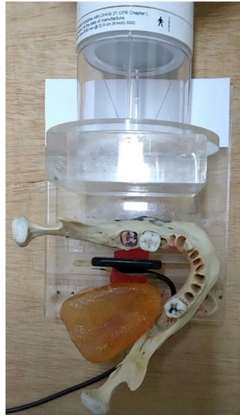
Fig. 2. An acrylic device used for image acquisition standardization and soft tissue simulation, and the positioning of the digital receptor, with a coupled lead foil, between the mandible and tongue-shaped acrylic device. The digital receptor was positioned with the transversal long axis parallel to the tooth long axis.
