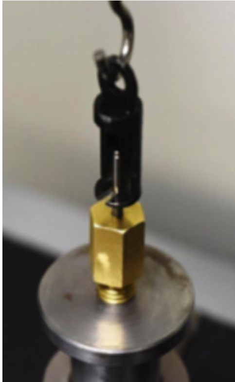
Fig. 5. Hitch/ hook positioned in the abutment neck to perform the traction test.
