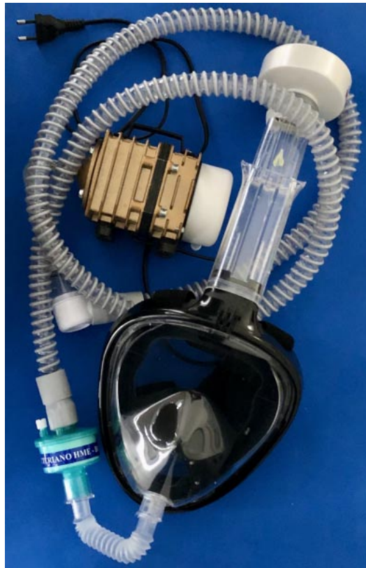
Fig. 3. Assembled air purifier system.
